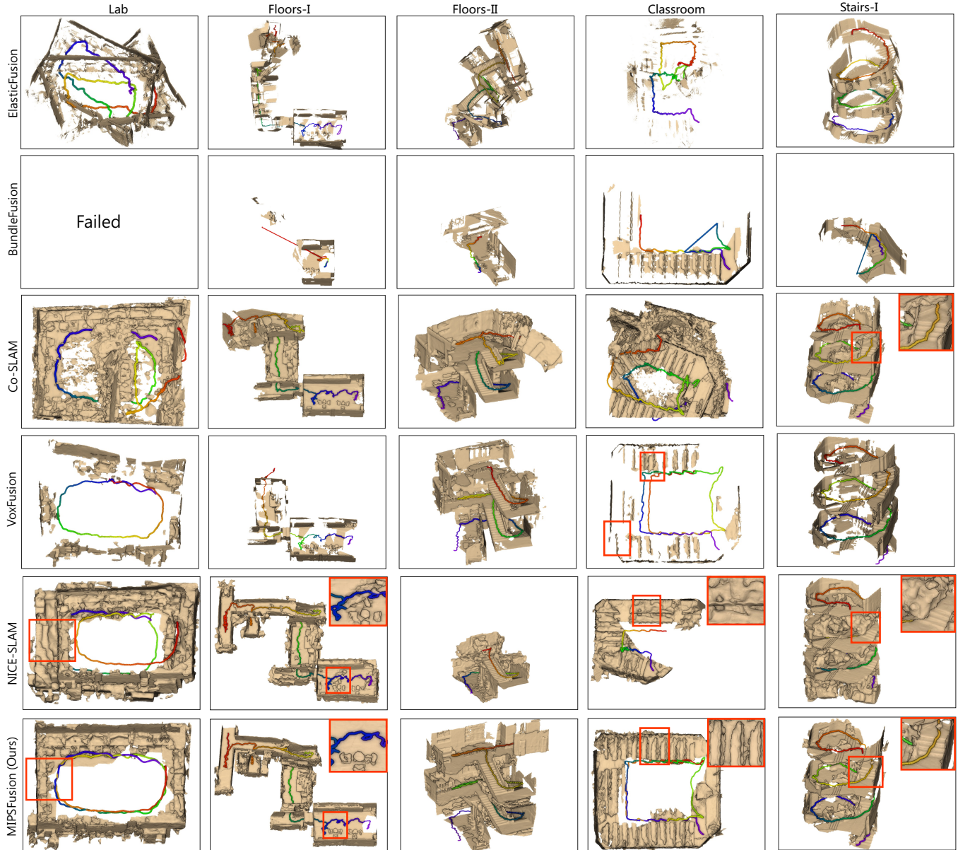
Fig. 16. Comparison of 3D reconstruction results by NICE-SLAM, Vox-Fusion, Co-SLAM, BundleFusion, ElasticFusion, and our MIPS-Fusion over five scenes from the FastCaMo–Large datasets. Our method achieves better accuracy and completeness compared to the alternatives.
